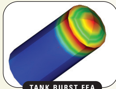
TANK BURST FEA
